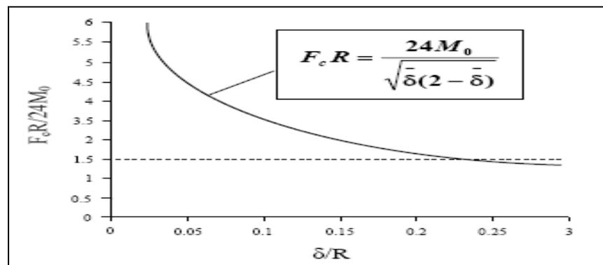
Figure 4. Ring crushing force  $F_c$  plotted with indent depth  $\delta$
