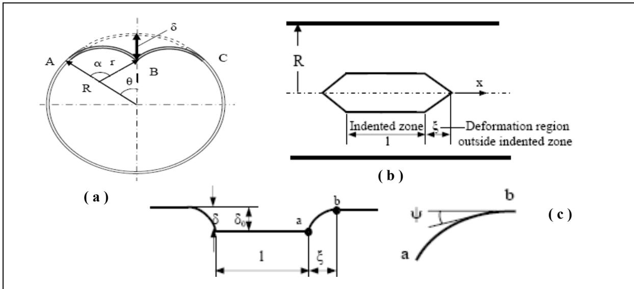
**Figure 2. (a) Deformation shape of ring, (b) Plan view of deformation region
