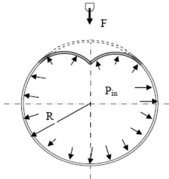
Figure 5. Deformation of a pressurized pipe
