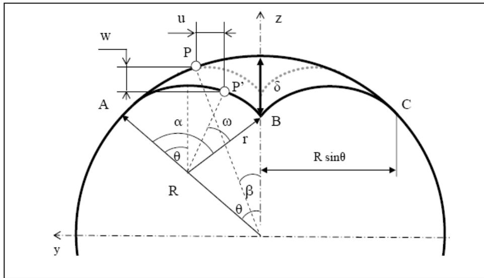
**Figure 3. Deformation region on ring section**
