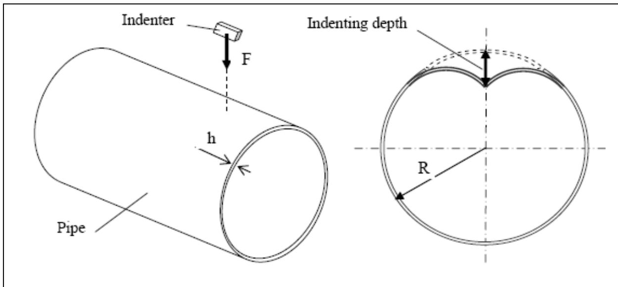
**Figure 1. Deformation shape of pipe and ring subjected to impact**
