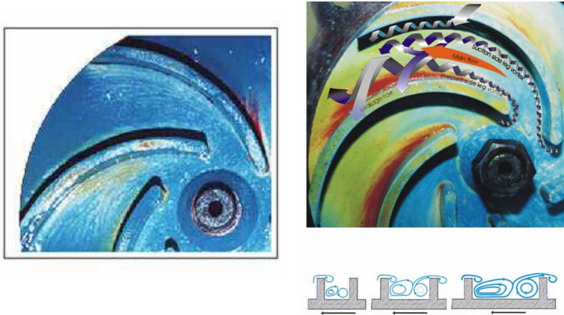
Figure 3-4. Flow pattern in impeller 30-40 (left) and impeller 30-20 (right)
