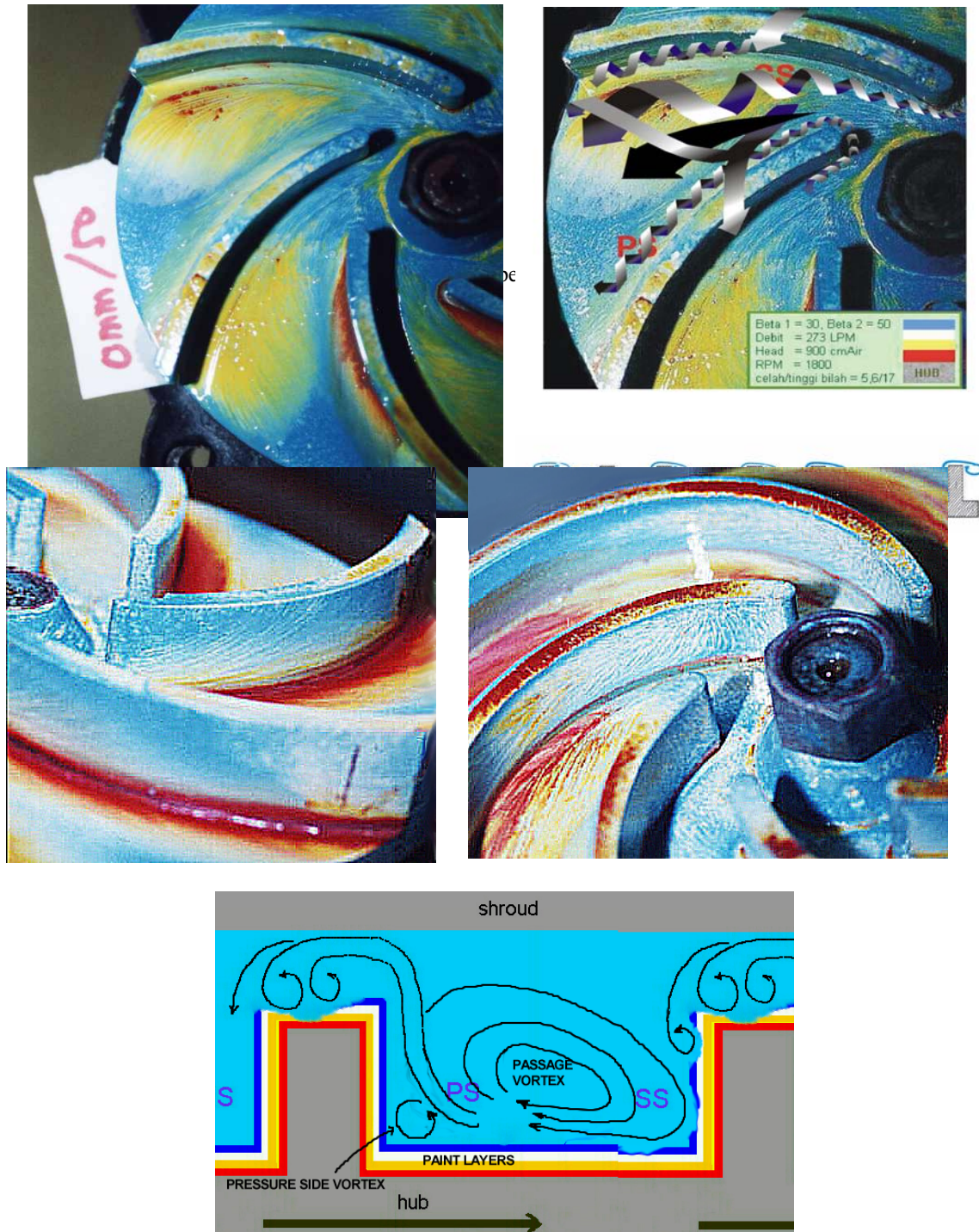
Figure 3-2. Flow pattern on the wall of pressure side (a), on the wall of suction side (b) and their interpretation (c)
