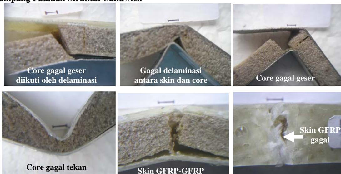
Gambar 7. Penampang patahan uji impact.
