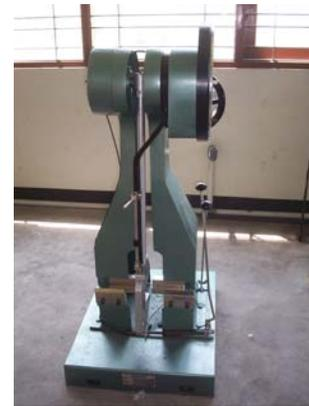
Gambar 4. Alat uji impak charpy
