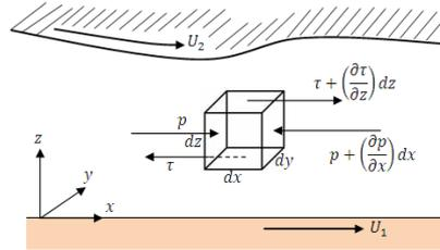
**FIGURE 1:** *Equilibrium of viscous shear forces and pressure forces, reproduced from [2].*
