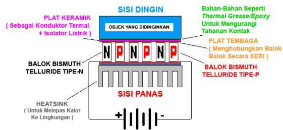
Gambar 1. Skema Modul Termoelektrik Sumber: Melcor Industries, ( www.melcor.com )
