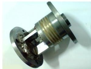
**Gambar 6.** Torque sensor
