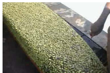
Gambar 1. Kapal model lambung kasar
