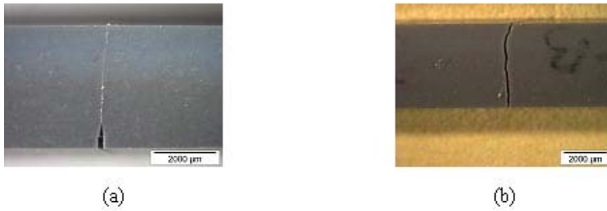
Figure 3. Valid crack propagation from SEVNB method (a). Valid crack propagation from SCF method (b)
