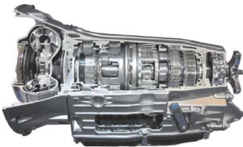
Figure 2. Automatic transmission (AT) named “7G-Tronik” from Mercedes-Benz
