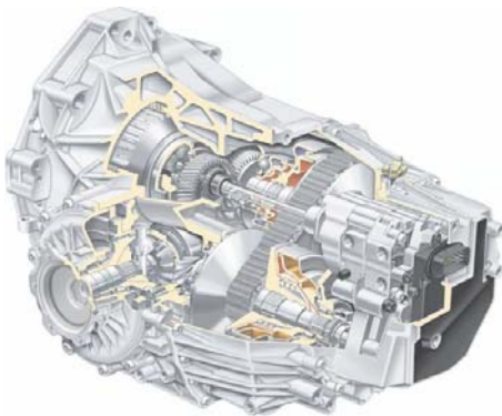
Figure 5. CVT named “multitronic” from Audi which Installed
