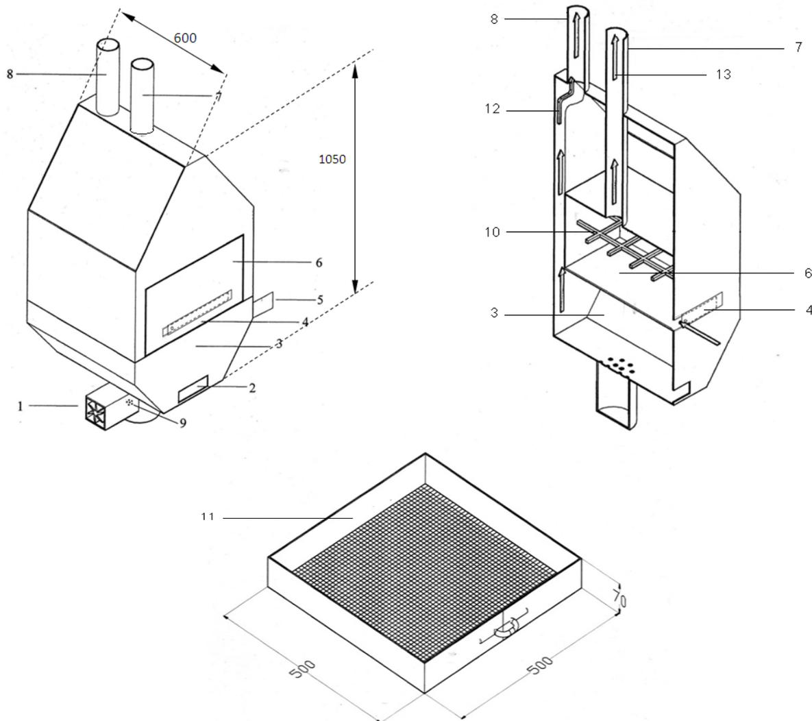
Figure 2. The drier designed for experimental purposes
