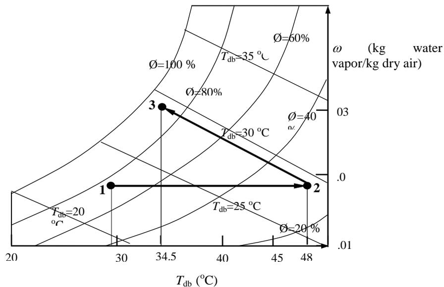
Figure 1. Paths on psychrometric chart illustrating heating and drying processes
