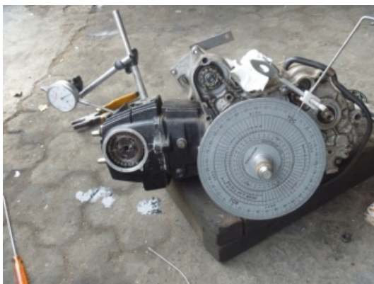
Gambar 1. Cam degreeing dial test
