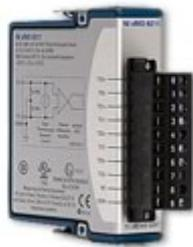
Gambar 3.9 Data akuisisi NI cDAQ-9172 Compact DAQ Chassis dan NI 9211 4-Channel, 14 S/s, 24-Bit,  $\pm 80$  mV Thermocouple Input Module
