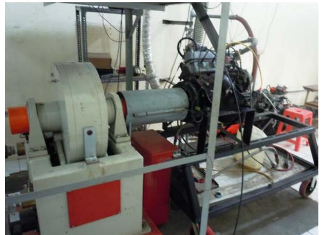
**Gambar 3.** Engine Test Bed Dynamite dan motor bakar bensin (Otto)
