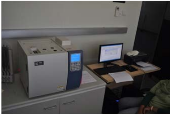
Gambar 4. Foto alat ukur kadar gas hydrogen (H 2 ), chromatography analyzer.
