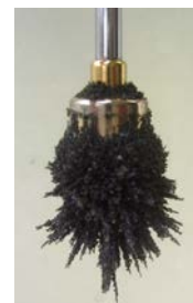
Figure 1. Iron sands from south coast Bantul Yogyakarta attached to permanent magnet.
