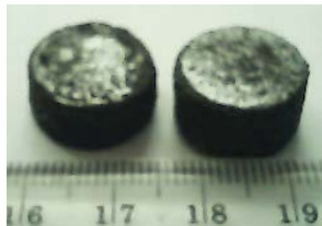
Figure 3. Sintered product magnet from iron sand
