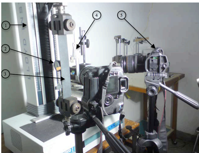
Figure 2. Experimental Setup (1) universal testing machine, (2) dial-gage, (3) specimen, (4) millimeter ruler, (5) camera.
