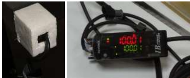
Figure 4. Laser beam sensor equipped with amplifier and power supply system.
