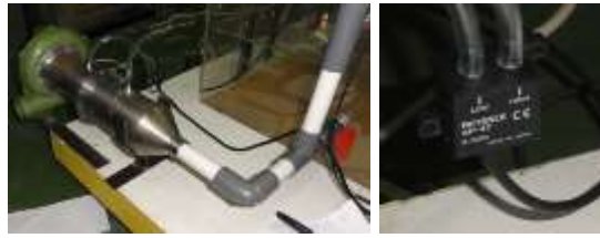
Figure 3. Orifice meter equipped with differential pressure measurement and amplifier system.
