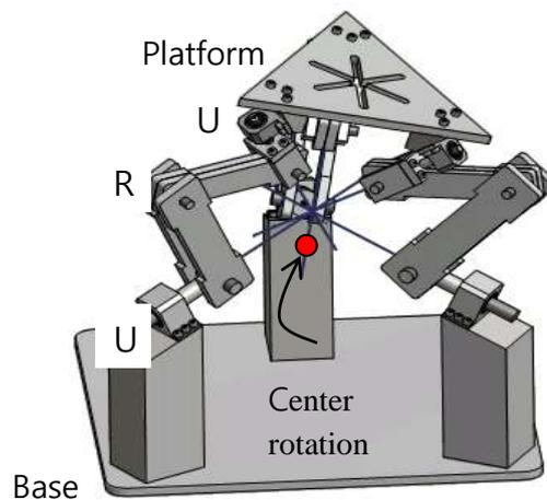
**Figure 4.** Cad diagram of 3-URU spherical parallel mechanism
