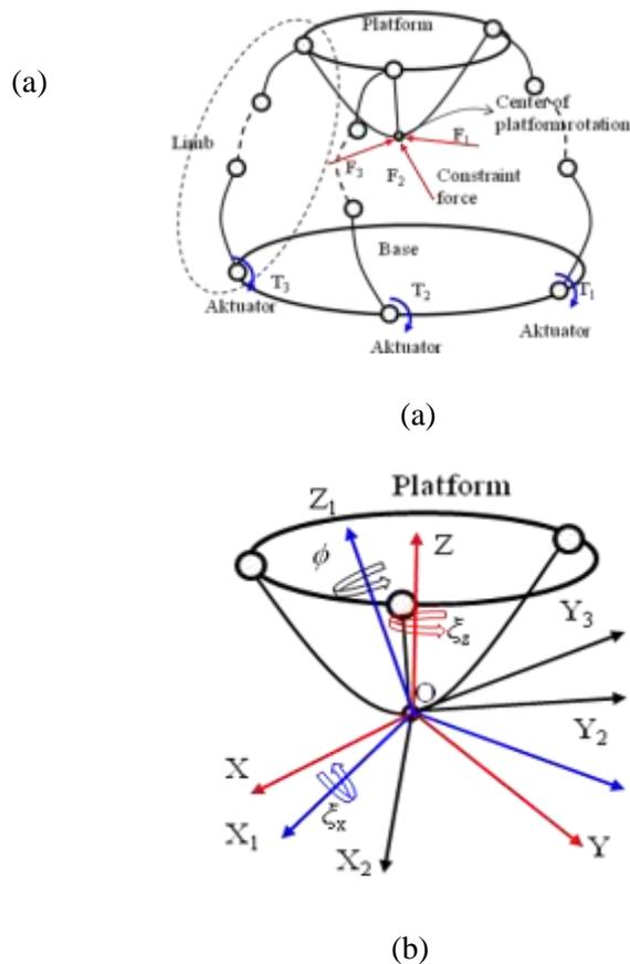
**Figure 1.** 3-dof spherical platform motion
