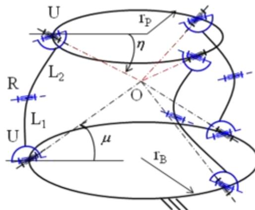
**Figure 3.** 3-URU spherical parallel mechanism
