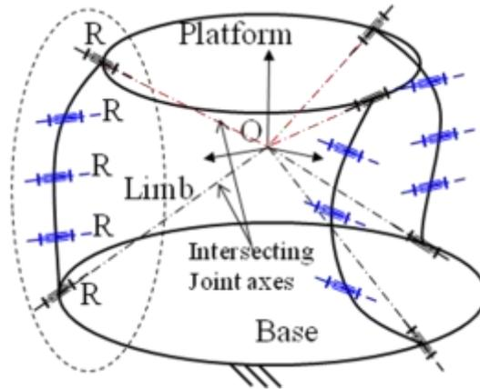
**Figure 2.** 3-5R spherical parallel mechanism
