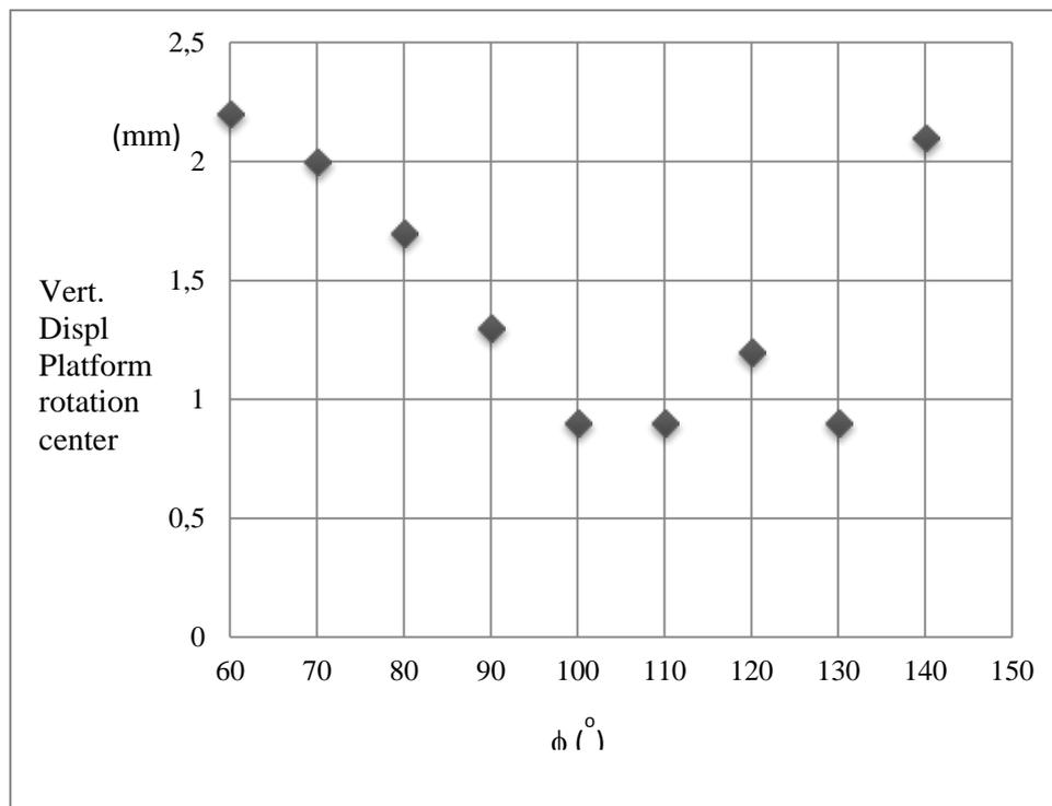
Figure 6 Displacement of the center of platform rotation for various  $\phi$  ( $W = 8 \text{ Kg}$ )
