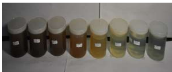
Figure 4. Change in color and turbidity of batik waste with Ethanol after 2, 4, 6, 8, 10 and 12 minutes flotation for 15 Volt bubble generator
