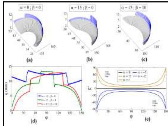
**Figure 6.** Geometry of cut (a) Test 1, (b) Test 2, (c) Test 3, and (d) the length of cut for CC-37, (e) Effect of inclination angle on toroidal angle of LE-point
