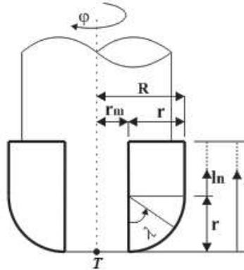
Figure 2. Geometry of toroidal cutting tool
