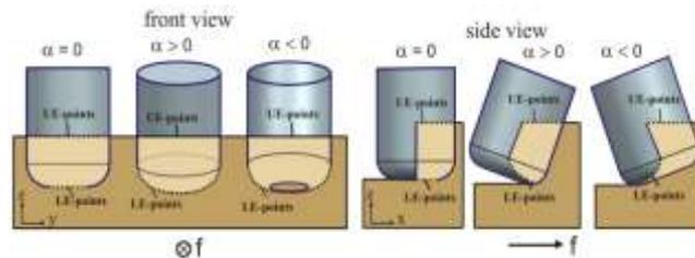
Figure 4 Effect of inclination angle to LE-point
