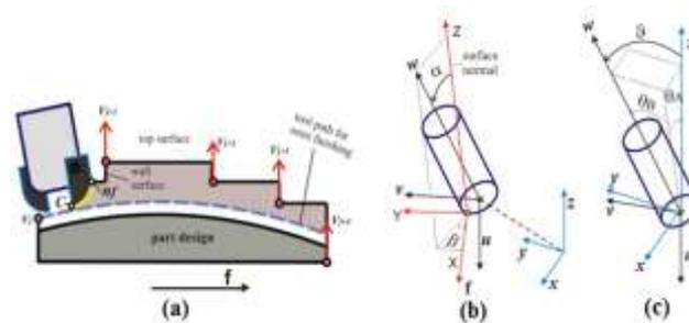
**Figure 1.** (a) Typical of workpiece surface from rough milling; illustration of the coordinate system, (b) three coordinate frame, (c) tool orientation relative to WCS
