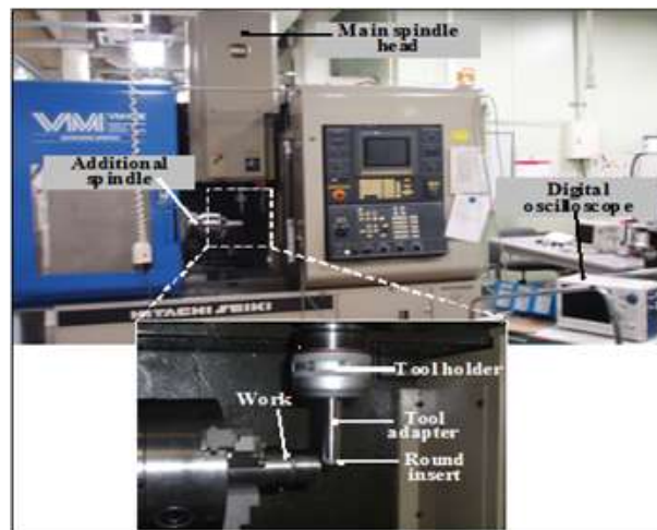
Figure 2. Photograph of experimental equipment of the vertical machine center (Harun, 2011)
