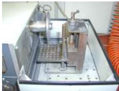
Figure 5. Initial V-Notching Process by using diamond wheel
