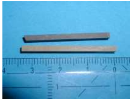
Figure 8. The accurate size of the specimens for fracture toughness tests of advanced ceramic
