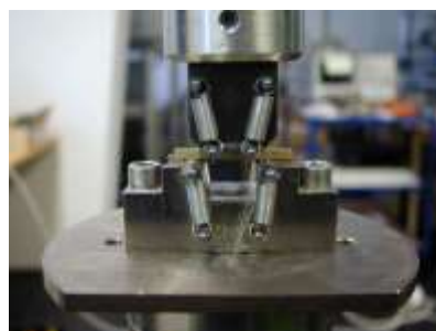
Figure 6. Sharpening the notch tip by using razor blade with diamond paste
