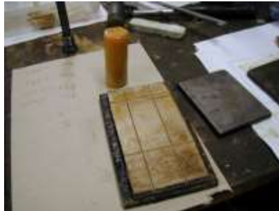
Figure 1. Ceramic tile on steel plate for mounting the samples. The sample was glued on the surface of the ceramic tile. The steel plate will hold by magnetic force.
