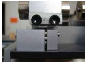
Figure 6. Sharpening the notch tip by using razor blade with diamond paste
