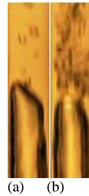
Fig. 4 Two different nose forms (a) U_{sl} = 0.77 m/s and U_{sg} = 0.22 m/s (b) U_{sl} = 0.77 m/s and U_{sg} = 0.55 m/s
