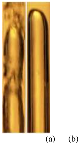
Fig. 3 Two different shapes of the plug (a) U_{sl} = 1.1 m/s and U_{sg} = 0.22 m/s (b) U_{sl} = 0.44 m/s and U_{sg} = 0.22 m/s
