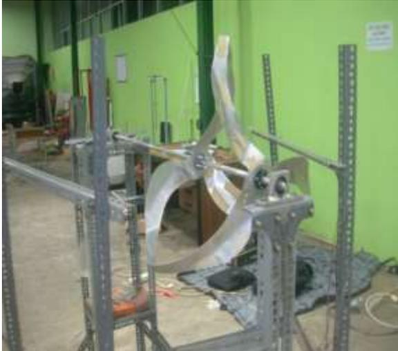
Gambar 1. Model Turbin Bersudu Loopwing
