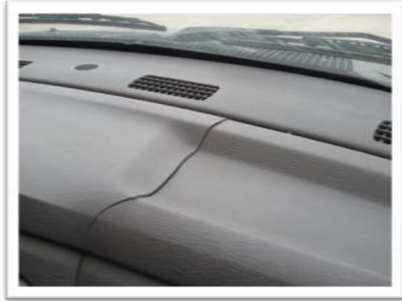
Figure 4. Cracked Dashboard Due to High Temperature Inside Car Cabin.
