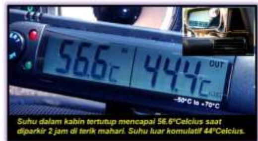
Figure 2. Car cabin temperature and ambient temperature
