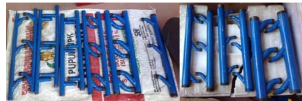
Gambar 6. Variasi diameter pipa header
