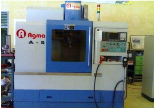
Gambar 1. Mesin Milling CNC Agma A-8
