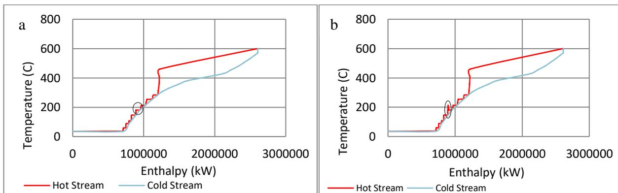
Figure 6 Composite Curve Diagram: (a) OFWH modeled as CFWH and (b) OFWH modeled as OFWH
