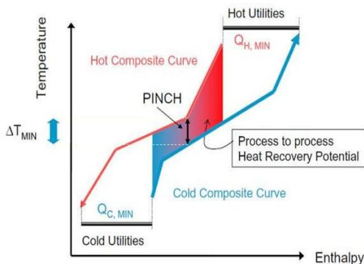
Figure 3 Composite Curve [5]
