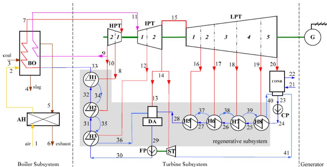
Figure 1 Supercritical power plant diagram. [3]
