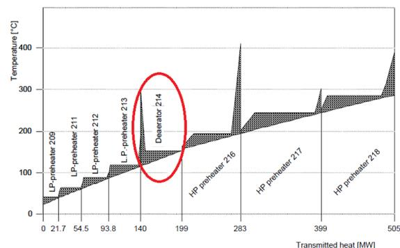
Figure 4 Composite curve of steam power plant [12]
