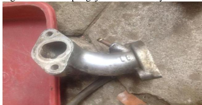
Gambar 5. Intake Manifold Standar
