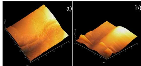
Figure 4. 3D Surface topography resulting from Universal Scanning Probe Microscopy (USPM): (a) hybrid 450°C (b) 500°C samples
