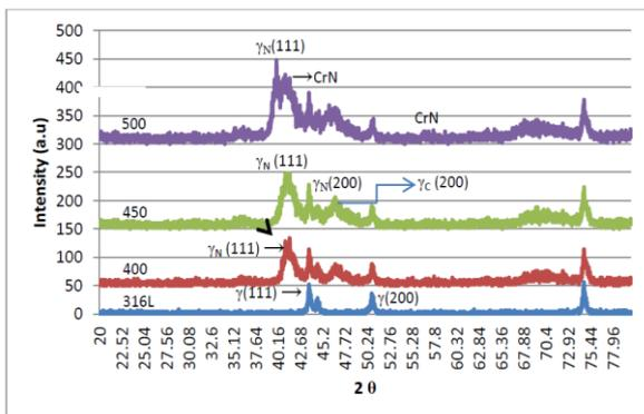
Figure 3. Comparison of XRD patterns of hybrid treated specimens from 400 °C to 500 °C as compared to untreated 316L
