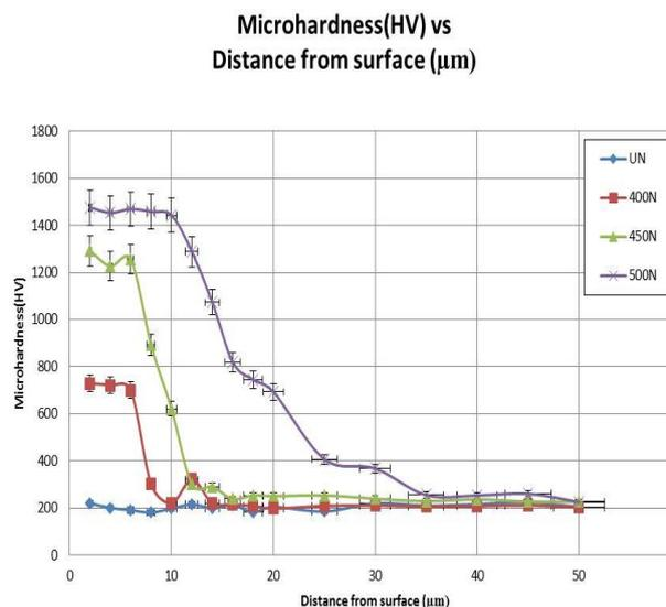
Figure 1. Microhardness depth profile
