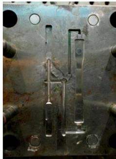
Gambar 3. Mold specimen uji tarik
