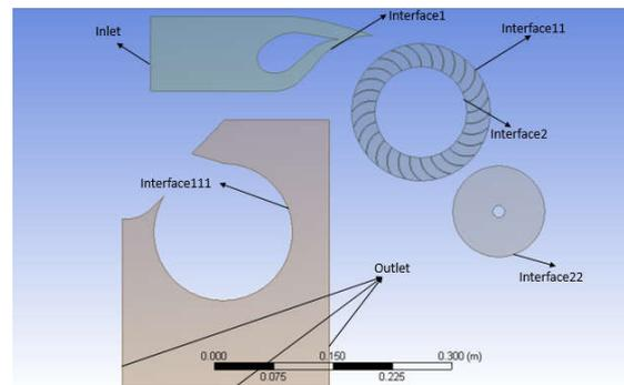
Figure 10. The Interface naming for each selected interface of the geometry parts
