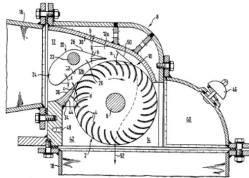
Figure 4. Control flow vane patent by Ossberger [3]
