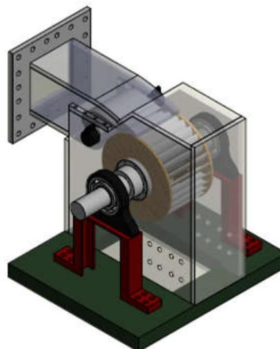
**Figure 19.** 3-D Model of the designed CFWT Turbine for experiment
