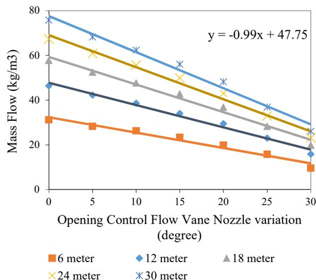
**Figure 18.** Graphic of mass flow to the opening Control Flow Vane Nozzle variation
