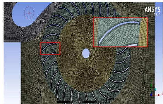
Figure 11. The Boundary Layers and mesh on each blades of the turbine runner
