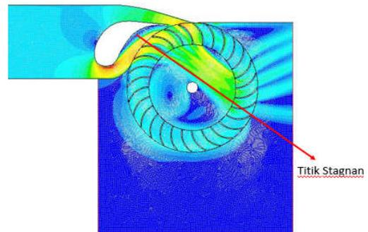
Figure 1. Control flow vane nozzle design initial design with unwanted stagnation point
