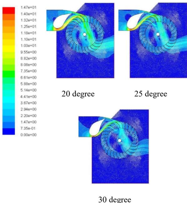
**Figure 17.** Velocity magnitude contour of opening Control Flow Vane Nozzle variation
