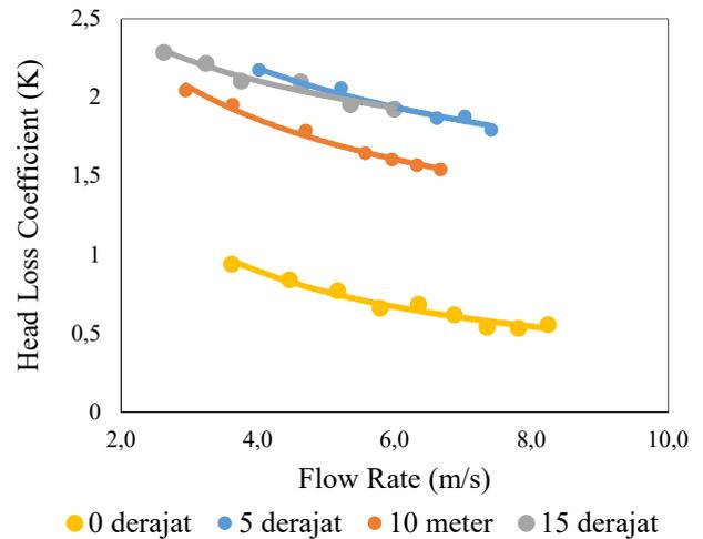
**Figure 16.** Graphic of head loss coefficient on opening Control Flow Vane Nozzle variation
