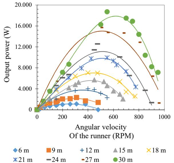
**Figure 13.** Graphic Output Power vs Angular Velocity of the Runner (RPM) with full opening Control Flow Vane Nozzle
