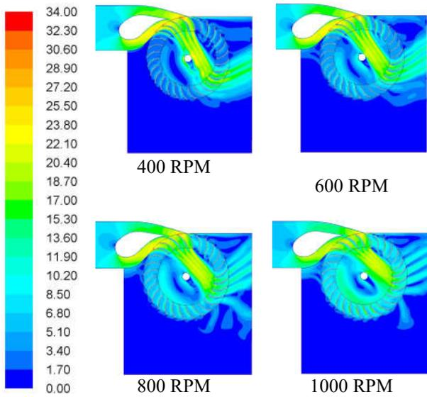
**Figure 14.** Velocity magnitude contour of Control Flow Vane Nozzle with 30 meters head
