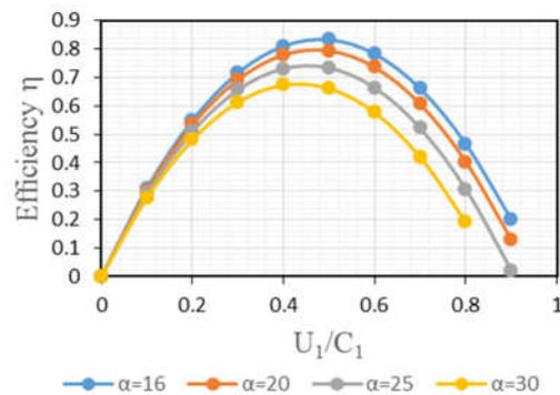
Figure 2. Cross Flow Turbine efficiency for each Angle of Attack
