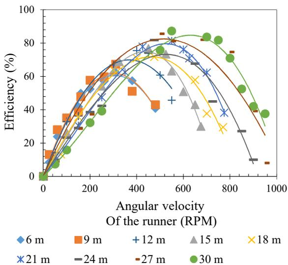
**Figure 12.** Graphic Efficiency vs Angular Velocity of the Runner (RPM) with full opening Control Flow Vane Nozzle
