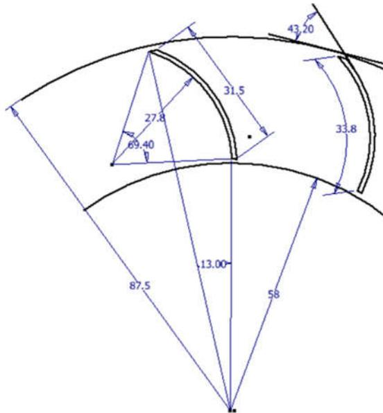
Figure 3. Geometry details configuration of the designed CFWT Turbine
