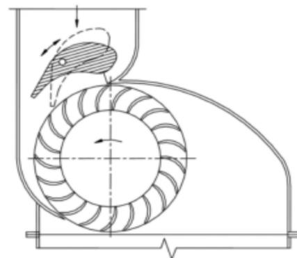
Figure 6. Control flow vane design by L.A.M.HI [4]
