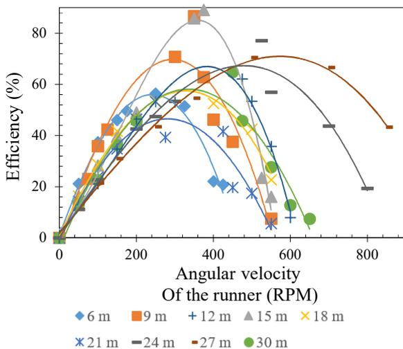
**Figure 15.** Graphic Output Power vs Angular Velocity of the Runner (RPM) with 5 degrees opening Control Flow Vane Nozzle
