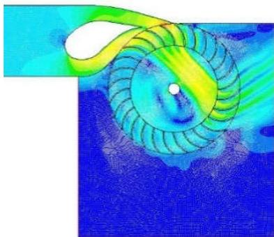
Figure 8. Control Flow Vane Nozzle final design with laminar flow
