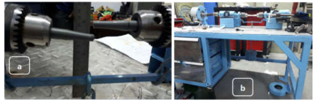
Figure 6. (a) The specimen is broken in the middle of the specimen length, and (b) the construction of the fatigue test machine from the front view
