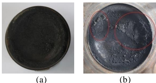
(a) (b) Gambar 2. Endapan terbentuk di head piston (a) Arak bali, (b) premium.
