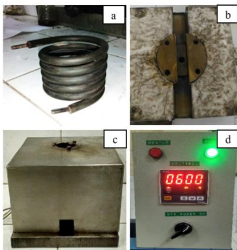
Gambar 7. Heater dan Controller a). Coil Heater , b). Glass wool c). Cover heater , d). Controller
