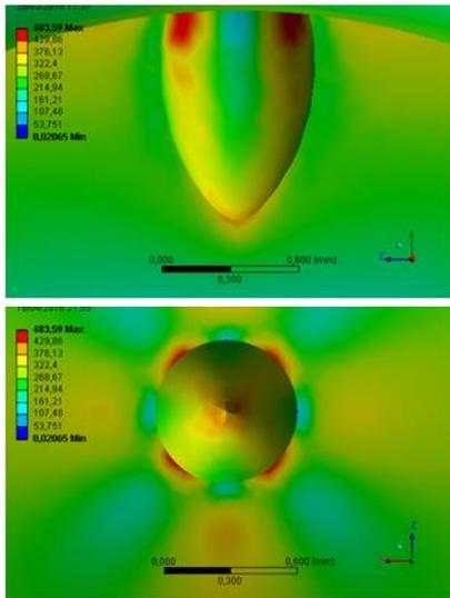
Figure 5 Stress distributions on narrow-deep pit (side and top view)
