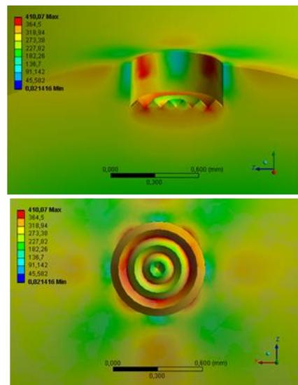
Figure 3 Stress distributions on vertical grain attack pit (side and top view)
