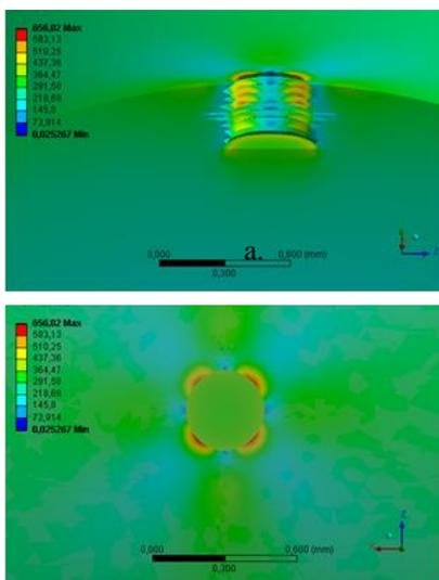
Figure 7 Stress distributions on horizontal grain attack pit (side and top view)
