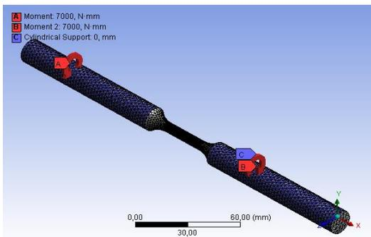
**Figure 1** Geometry and boundary condition of finite element model
