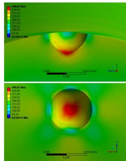
Figure 4 Stress distributions on elliptical pit (side and top view)
