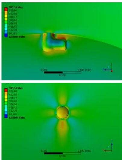
Figure 6 Stress distributions on undercutting pit (side and top view)
