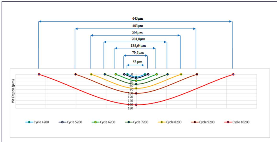
**Figure 12** The evolution of pit simulated
