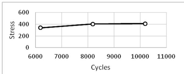
**Figure 13.** Maximum stress curve when pit growth occurred
