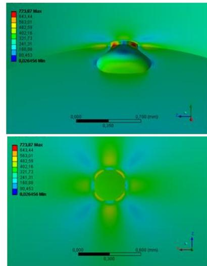
Figure 8 Stress distributions on subsurface pit (side and top view)
