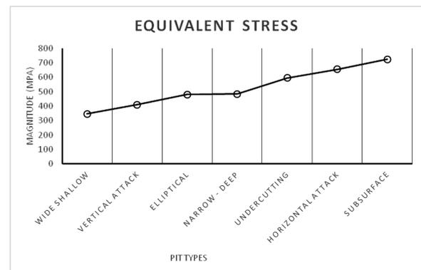
Figure 9 Comparison of equivalent stress magnitude on different types of pit
