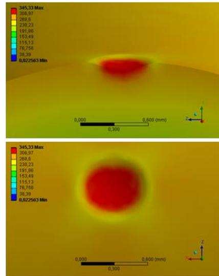
Figure 2 Stress distributions on wide shallow pit (Side and top view)
