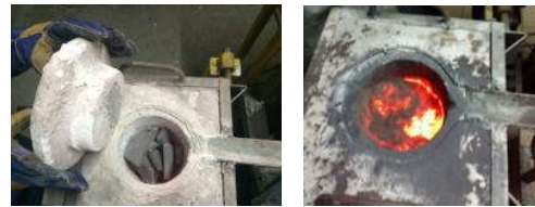
Gambar 2. Proses peleburan aluminium.
