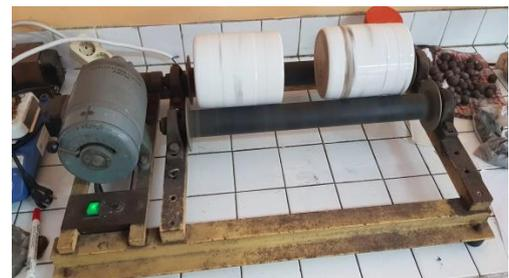
Gambar 3. Ball Mill Motor Listrik
