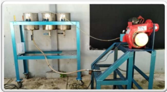
Gambar 6. Setting eksperimen burner simulator
