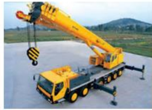
b. Mobile Crane
