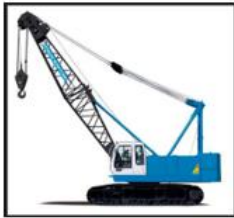
a. Crawler Crane
