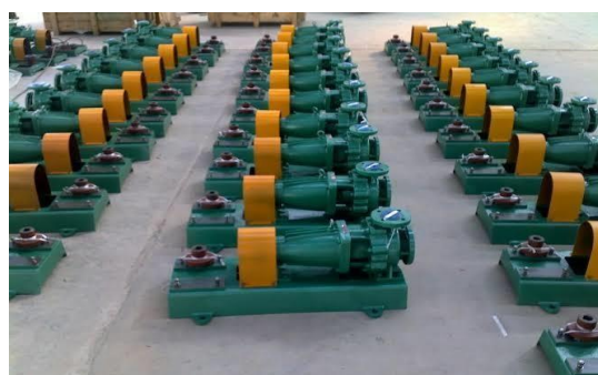
Gambar 4.6 pompa IHF fluorine plastic alloy single stage single suction kimia pompa sentrifugal.
