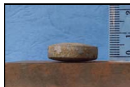
Gambar 4. Sampel Hasil Sinter 900°C
