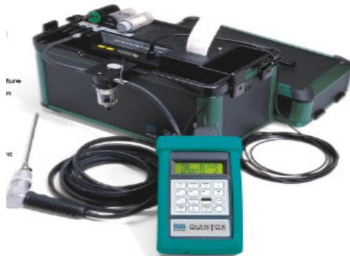
Gambar 3. Quintox Flue Gas Analyzer
