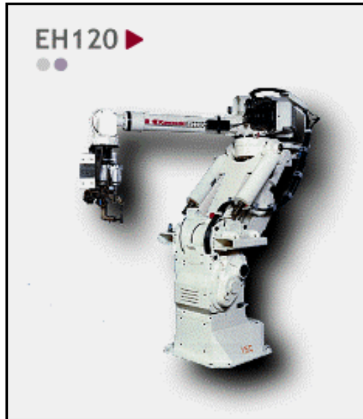
Gambar 1 : Robot Kawasaki EH 120, payload =120 kg
