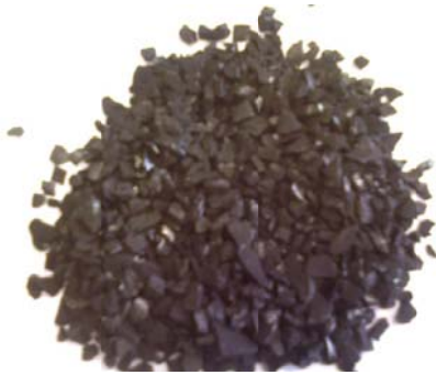
Figure 2. Photo of flake active carbon (filler) from Palm Waste
