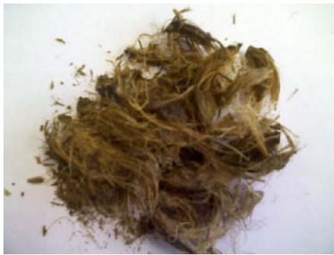
Figure 3. Photo of Palm Kernel Shell Fibers
