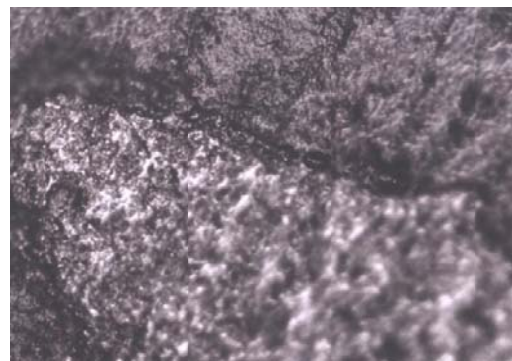
Figure 8. Microstructure of sample(X150). Showing interface between matrix and fiber.
