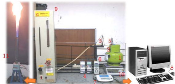
Gambar 5. Skema pengujian hubungan antara laju aliran dengan tekanan keluar regulator; (1)Tabung gas LPG 3 kg; (2)Regulator; (3)Pressure transducer; (4)Pressuremeter; (5)Termokopel; (6)Termometer digital; (7)Data akuisisi RS232; (8)Komputer; (9)Rotameter; (10)Timbangan; (11)Bunsen burner
