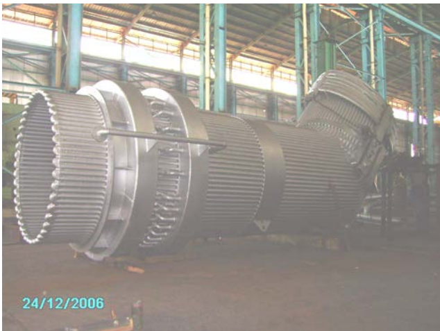
Gambar 2. Water-cooled hot gas duct section 1 (Sumber: PT. Krakatau Steel, 2008)
