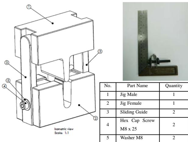
**Figure 1 (a)** A special bending jigs which were used to stress the cold-rolled samples; and **(b)** The actual size of the U-bend sample.
