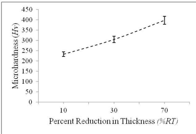
**Figure 6.** Microhardness values of the cold-rolled 316L stainless steel
