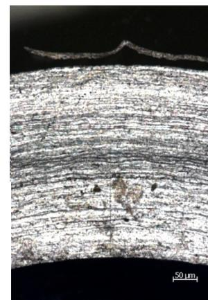
**Figure 10** Surface morphology of the U-bend sample after 70% cold deformation at the maximum bending region (magnifications of 100x).
