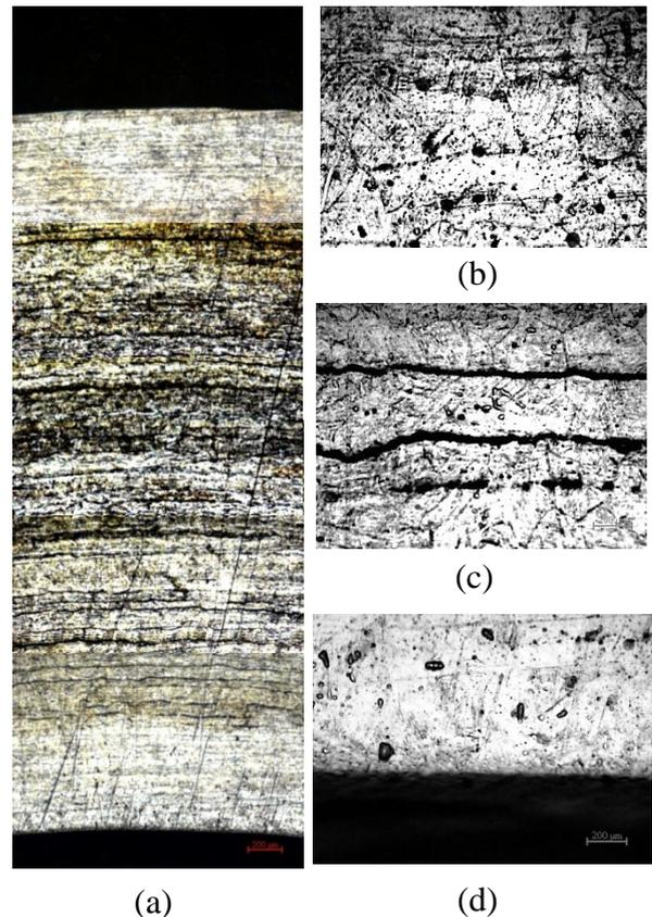
**Figure 8** Surface morphology of the U-bend sample without cold rolled process at (a) the maximum bending point (magnifications of 100x); (b) top; (c) center and (d) bottom region (magnifications of 500x).
