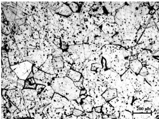
**Figure 2.** Optical micrograph of the as-received 316L stainless steel (magnifications of 200x).
