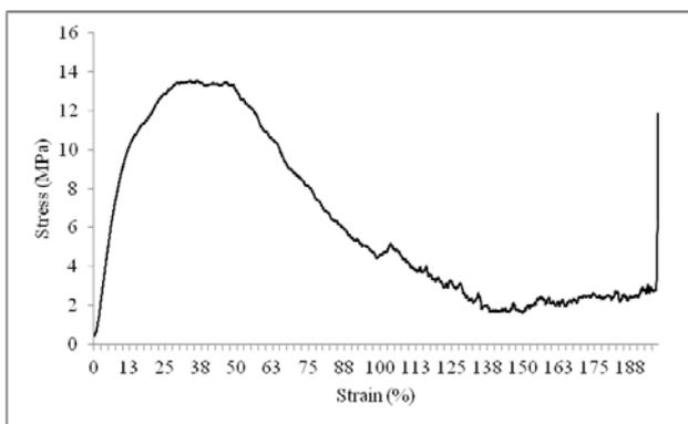
**Figure 7.** The stress-strain curve of the U-bend samples after 70% thickness reduction.
