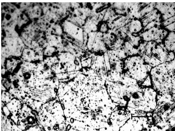
**Figure 3.** Optical micrograph of the cold rolled 316L stainless steel after 10 % thickness reduction (magnifications of 500x).
