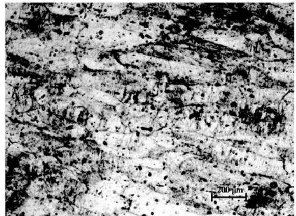
**Figure 5.** Optical micrograph of the cold rolled 316L stainless steel after 70% thickness reduction (magnifications of 200x).
