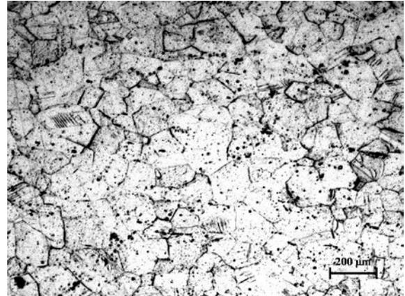
**Figure 4.** Optical micrograph of the cold rolled 316L stainless steel after 30% thickness reduction (magnifications of 200x).
