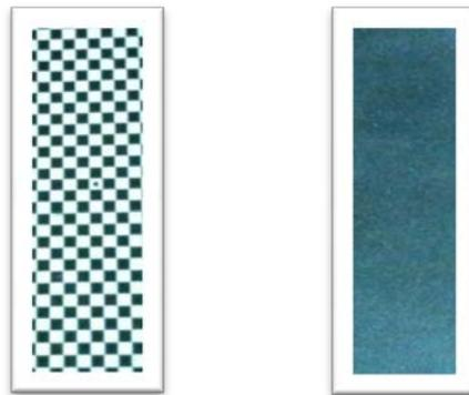
**Figure 3.** Experimental object: calibration board (left), speckled-specimen (right).
