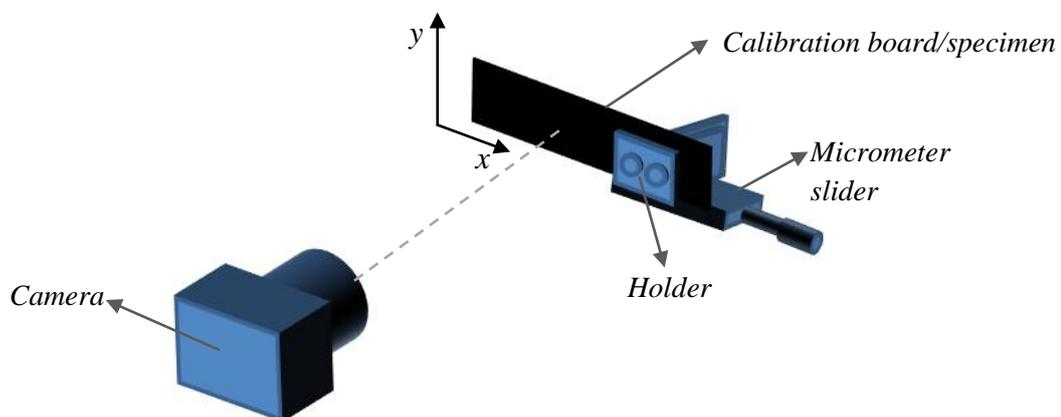
**Figure 4.** Schematic of the experimental setup.
