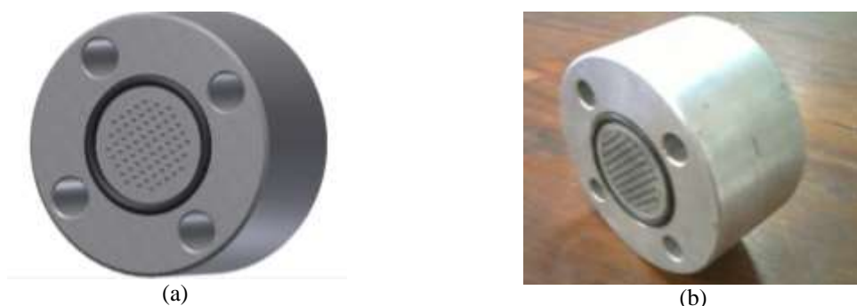
Figure 2. Porous media casing (a) computer design, (b) real model
